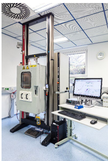
Picture 2: Tensile testing machine with 80 °C heated chamber for SHT
