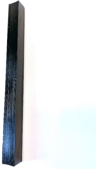
Picture 6: FNCT test specimen prepared with notch before testing
