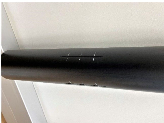
Picture 1: Pipe specimen prepared with 4x notches for the NPT or ANPT test
